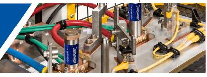
The VeriFast™ IA (Integrated Amplifier) Nut Detection Solution is CenterLine's latest system for monitoring weld pin position, an important part of the projection welding process.
